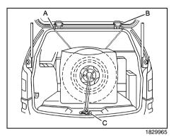
5) Pull the cable (A) through the door striker (C) and the center of the wheel.
